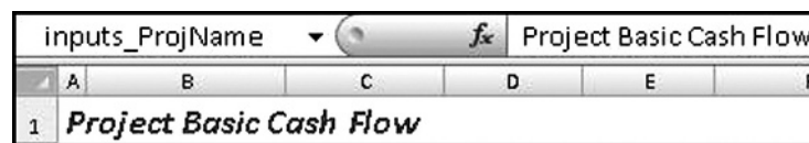
FIGURE 1.7 In cell A1, on the Assumptions sheet, we create a label for the cell by entering text. Notice the cell is also named, as seen by the name inputs_ProjName in the Name Box.
