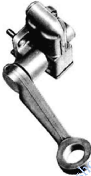
Figure 1.1.19 The simple lever-arm damper can be reinforced to carry suspension loads by lengthening the bearing rod.
