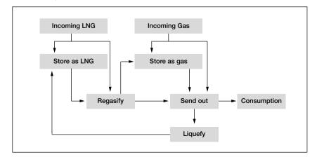
is injected into a special underground natural gas storage facility (onshore or offshore), to be redelivered at a later date when market demands dictate. This is the essence of gas storage, which is a means of holding a gas inventory for release into an energy market when it is most needed.
