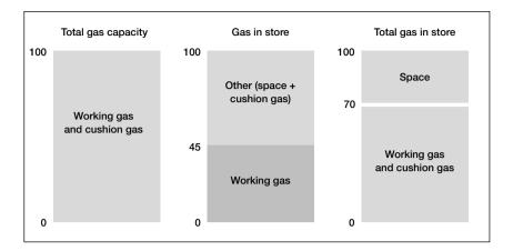
A larger volume gas storage project will inevitably have a longer duration, but this is not an absolute measure of performance – as a rule of thumb, doubling the rate of deliverability will halve the duration, and halving the rate of redelivery will double the duration.
